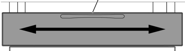
**1 Side to Side:** Rotate all barrels in the direction you want the drawer face to move.
