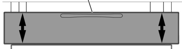
**2 Up and Down:** Slide the gray tab on the side to be moved. Slide the tab toward the back of the drawer to raise the drawer face.
