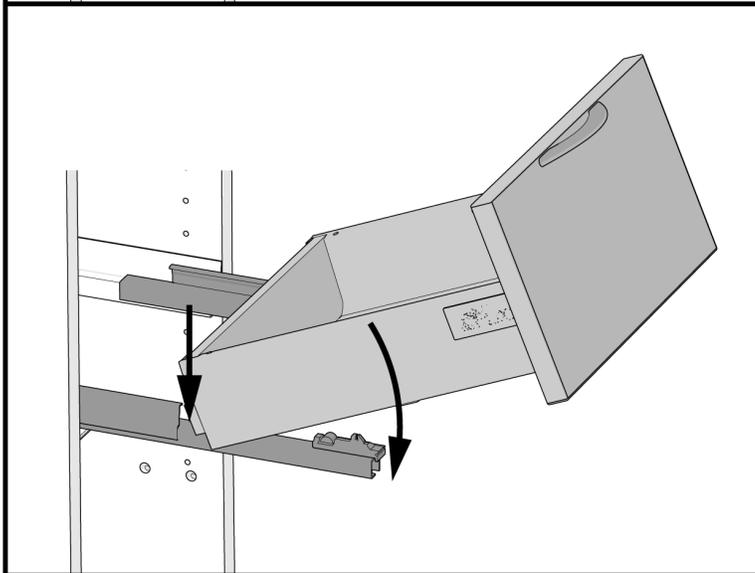
**2** Align the drawer with the extended slides then insert the drawer onto the slides.
