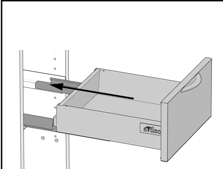
**3** Push the drawer in and ensure that it is engaged with both slides. Confirm the drawer moves smoothly through its full range of motion.
